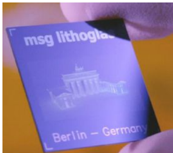
structured and transparent Lithoglas® coatings, e.g. for the packaging of optical devices
