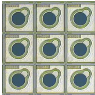
structured and transparent Lithoglas® coatings, e.g. for the packaging of optical devices
